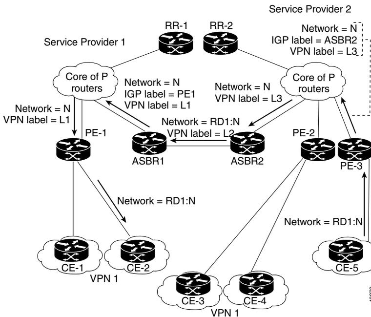
Figure 5 shows the same packet forwarding method as described in Figure 4, except the EBGP router (ASBR1) forwards the packet without reassigning it a new label.
