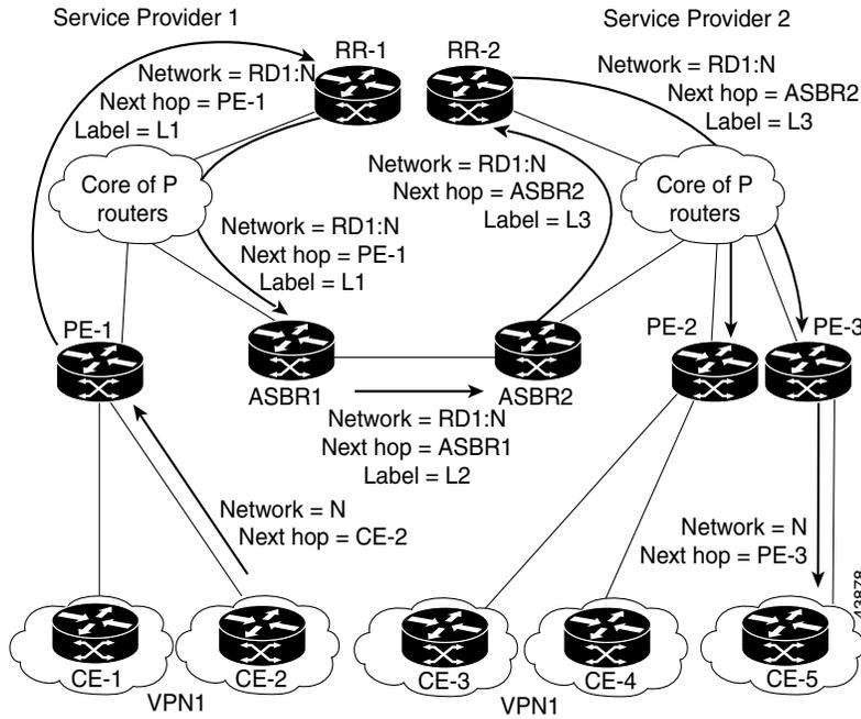
Figure 3 illustrates the exchange of VPN route and label information between autonomous systems. The only difference is that ASBR2 is configured with the **redistribute connected** command, which propagates the host routes to all PEs. The **redistribute connected** command is necessary because ASBR2 is not configured to change the next-hop address.
