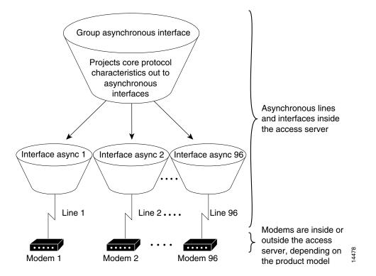
Use the **interface group-async** command to create and configure a group asynchronous interface. The following example shows a group asynchronous configuration for a Cisco AS5300 access server loaded with one 4-port ISDN PRI card and 96 MICA modems:
