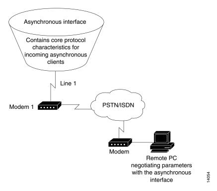
To enable clients to dial in, you must configure two asynchronous components: asynchronous lines and asynchronous interfaces. Asynchronous interfaces correspond to physical terminal lines. For example, asynchronous interface 1 corresponds to tty line 1.
