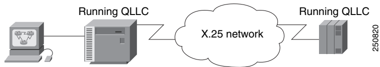
Figure 9 SNA Devices Running QLLC
