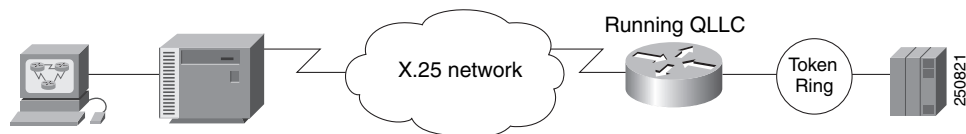
Figure 10 Router Running QLLC Conversion Feature
