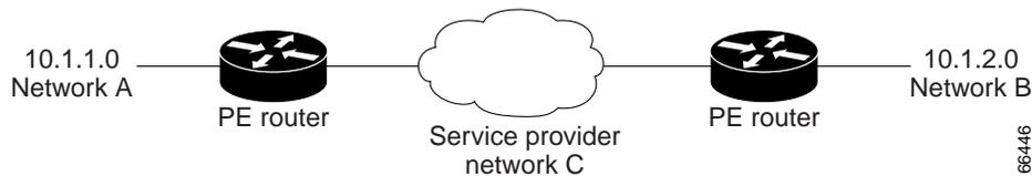
**Figure 1** shows a high-level view of a GRE tunnel in a service provider network. Traffic from device 10.1.1.0 in network A is sent through the provider network C to device 10.1.2.0 in network B. GRE tunneling allows networks A and B to appear to be directly connected. The only knowledge that the provider network has of the two customer networks is at the interfaces of the provider edge (PE) routers.
