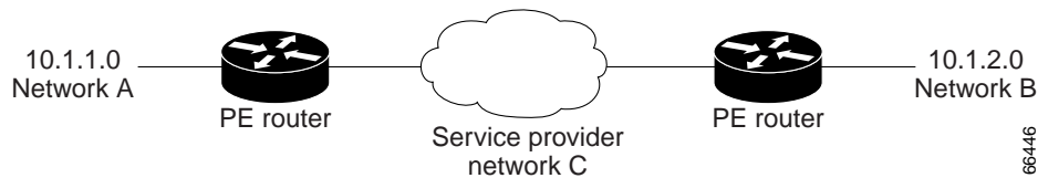
Figure 1 GRE Tunneling Between Provider Edge Routers
