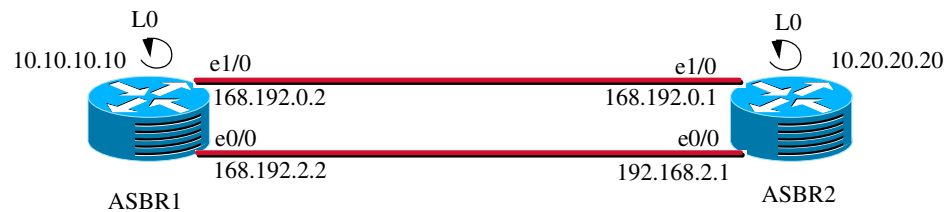
Figure 4 Loopback Interface Configuration for Directly-Connected ASBR1 and ASBR2 Routers
