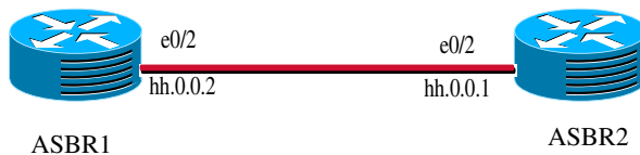
Figure 3 Configuration for Peering with Directly-Connected Interface Between ASBRs
