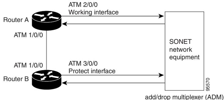
On the protect circuit, the K1 and K2 bytes from the line overhead (LOH) of the SONET frame indicate the current status of the APS connection and convey any requests for action. This signalling channel is used by the two ends of the connection to maintain synchronization.
