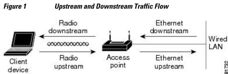
The radio downstream flow is traffic transmitted out the access point radio to a wireless client device. This traffic is the main focus for QoS on a wireless LAN.
