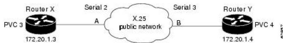
Figure 10 Establishing an IP Encapsulation PVC Through an X.25 Network
