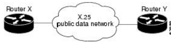
Figure 3 Transporting LAN Protocols Across an X.25 PDN
