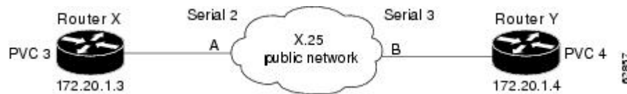
Figure 10 Establishing an IP Encapsulation PVC Through an X.25 Network
