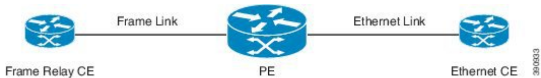
Figure 1: Frame Relay-Ethernet Local Switching Topology
