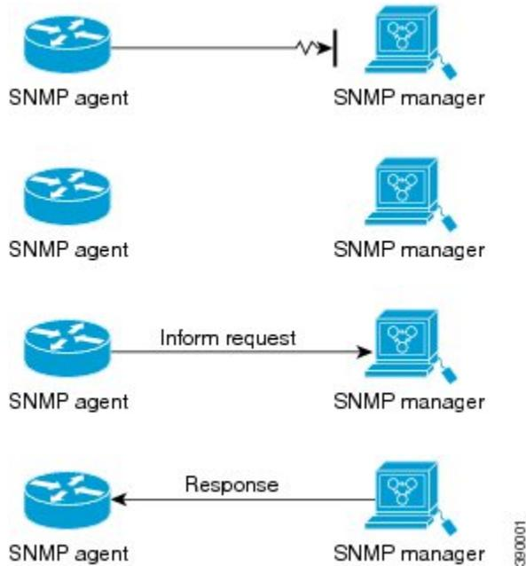
The figure below shows an agent sending a trap to a manager that the manager does not receive. The agent has no way of knowing that the trap did not reach its destination. The manager never receives the trap because traps are not resent.
