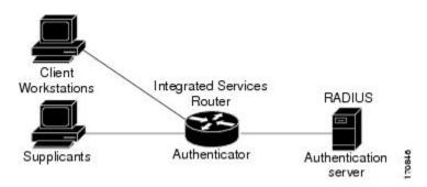
• Supplicant—Device (workstation) that requests access to the LAN and switch services and responds to requests from the router. The workstation must be running IEEE 802.1X-compliant client software such as that offered in the Microsoft Windows XP operating system. (The *supplicant* is sometimes called the client.)
