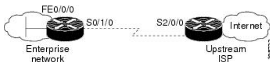
Figure 3: Enterprise Network Using Unicast RPF for Ingress Filtering
