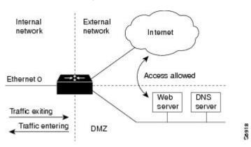
Using these two sample topologies, decide whether to configure CBAC on an internal or external interface.
