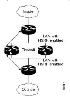
In a LAN WAN scenario, the inside interface of the Active Standby pair running the firewall are connected via LAN interface on the inside and WAN interface on the outside (see the figure below). HSRP is configured on the inside interface. The inside network communicates with the HA pair using the inside virtual IP address.
