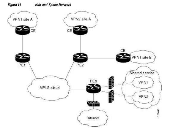
Typically each VPN has a VLAN and/or VRF subinterface connected to the Shared Service. When a packet arrives from an MPLS interface, the inner tag represents the VPN-ID. MPLS routes the packet to the corresponding subinterface that is connected to Shared Service.
