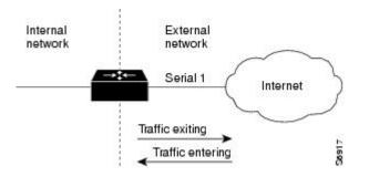
The second topology is shown in the figure below. In this topology, CBAC is configured for the internal interface Ethernet 0. This allows external traffic to access the services in the Demilitarized Zone (DMZ), such as DNS services, but prevents specified protocol traffic from entering your internal network--unless the traffic is part of a session initiated from within the internal network.
