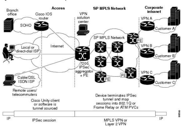
The figure below illustrates a scenario showing IPSec to MPLS and Layer 2 VPNs.
