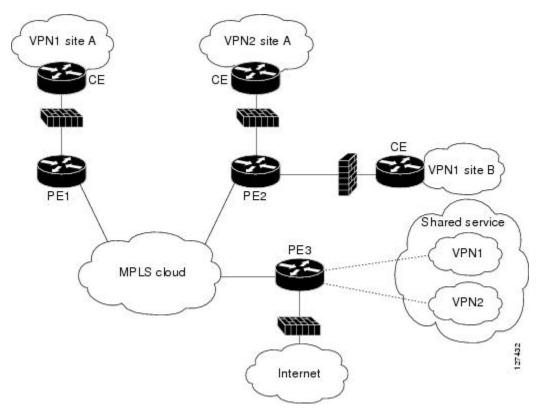
In this example, VPN1 has two sites, Site A and Site B, that span across the MPLS core. Site A is connected to PE1, and Site B is connected to PE2. VPN2 has only one site that is connected to PE2.
