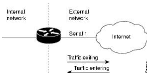
The second topology is shown in the figure below. In this topology, reflexive access lists are configured for the internal interface Ethernet 0. This allows external traffic to access the services in the Demilitarized
