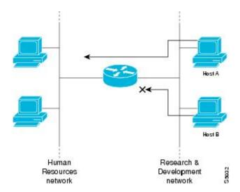
Access lists should be used in firewall routers, which are often positioned between your internal network and an external network such as the Internet. You can also use access lists on a router positioned between two parts of your network, to control traffic entering or exiting a specific part of your internal network.
