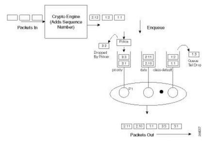
The image shows that the sequence number consists of two parts, namely the selector and the sequence number. The receiving side would use the selector to choose the correct history to use and the sequence number would operate as always.
