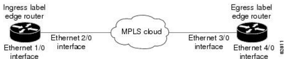
Figure 2 Network Topology for Mapping MPLS EXP Value
