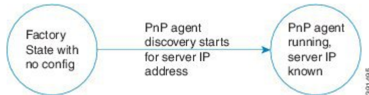
Figure 3: State Diagram for PnP Trigger with no Startup Configuration
