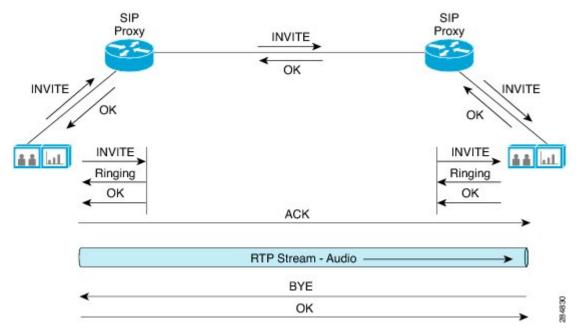
In the message exchange process for SIP, the INVITE message, which is used to establish a media session between user agents, carries SDP from the sender to the receiver. The associated SDP provides information about the bandwidth, the application name, and the sender port number. It also signals RTP, which is used as the protocol for communications.
