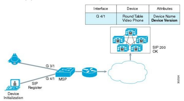
The SIP client, which is a round table video phone sends out SIP Register messages to the call manager. The call manager is responsible for routing the call across the enterprise network. Following sample packet capture highlights the UserAgent field in the SIP Register message, which identifies the device name and the device version.
