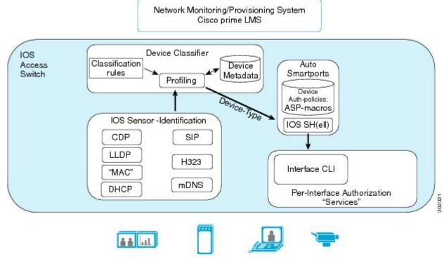
Based on the type of device identified, the physical interface to which the device is connected can be configured using auto smart ports with minimal configuration by network administrator. Based on the types of media flows identified, MSP provides services such as CAC and QoS to the network devices. The Device Identification, page 3 and Flow Identification Mechanisms, page 8 sections provide more information about the mechanisms used to identify devices and media flows.
