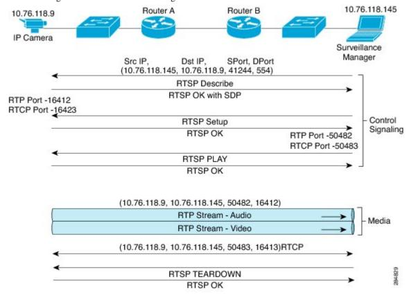
The client (which is the surveillance manager) sends a control request to the server (which is the IP camera), listing the source and destination IP addresses, and the source and destination port numbers.
