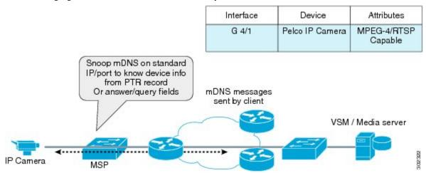
The figure shows an IP camera connected to the networking device (on which MSP is enabled). The IP camera sends mDNS messages to the multicast IP address 224.0.0.251 on standard mDNS port 5353. The networking device listens to these messages on the standard mDNS port and derives the device type and class. Based on these attribues, the device classifier looks up the best match and completes the profiling. Following is sample packet capture, which highlights the device name and class.
