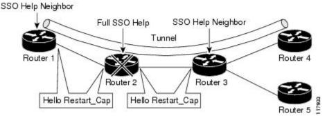
The Hello Restart\_Cap object has two values: the restart time, which is the sender's time to restart the RSVP\_TE component and exchange hello messages after a failure; and the recovery time, which is the desired time that the sender wants the receiver to synchronize the RSVP and MPLS databases.
