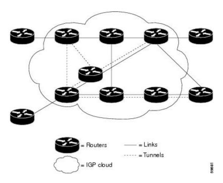
As a result, a TE tunnel is advertised as a link in an IGP network with the link's cost associated with it. Routers outside of the TE domain see the TE tunnel and use it to compute the shortest path for routing traffic throughout the network.
