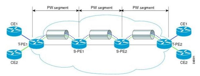
The end routers are called terminating PE routers (T-PEs), and the switching routers are called S-PE routers. The S-PE router terminates the tunnels of the preceding and succeeding PW segments in an MS-PW. The S-PE router can switch the control and data planes of the preceding and succeeding PW segments of the MS-PW. An MS-PW is declared to be up when all the single-segment PWs are up. For more information, see the *L2VPN Pseudowire Switching* document.
