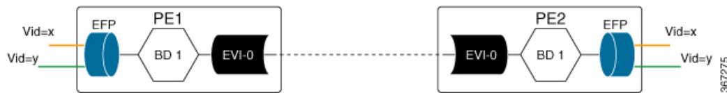
Figure 2: VLAN Bundle Service Interface
