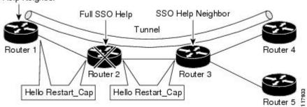
The Restart\_Cap object has two values--the restart time, which is the sender's time to restart the RSVP\_TE component and exchange hello messages after a failure; and the recovery time, which is the desired time that the sender wants the receiver to synchronize the RSVP and MPLS databases.
