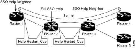
The Hello Restart\_Cap object has two values: the restart time, which is the sender's time to restart the RSVP\_TE component and exchange hello messages after a failure; and the recovery time, which is the desired time that the sender wants the receiver to synchronize the RSVP and MPLS databases.
