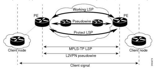
MPLS-TP is supported on ATM and TDM pseudowires on the Cisco ASR 903 router. For information, see Configuring the Pseudowire Class.
