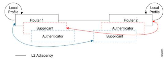
When the interface is configured for 802.1x role as both, The authentication manager on a router creates a session with two EAP session (blue and red with separate EAP session ID) flows with supplicant as well as an authenticator role and both trigger EAP-TLS mutual authentication with the local authenticating server.
