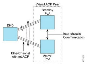
The PoAs forming a virtual LACP peer, from the perspective of the DHD, are defined as members of a redundancy group. For the PoAs in a redundancy group to appear as a single device to the DHD, the states between them must be synchronized through the Interchassis Communication Protocol (ICCP), which provides a control-only interchassis communication channel (ICC).
