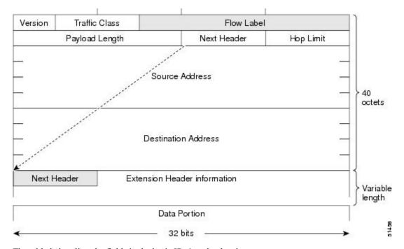
The table below lists the fields in the basic IPv6 packet header.
