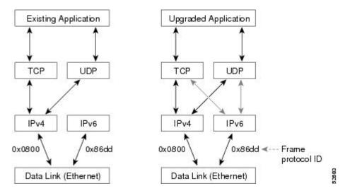
One application program interface (API) supports both IPv4 and IPv6 addresses and DNS requests. An application can be upgraded to the new API and still use only the IPv4 protocol stack. The Cisco software supports the dual IPv4 and IPv6 protocol stack technique. When an interface is configured with both an IPv4 and IPv6 address, the interface will forward both IPv4 and IPv6 traffic.
