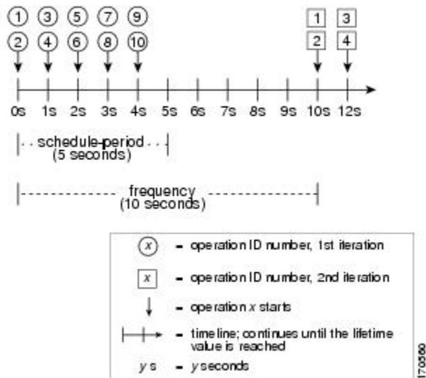
In this example, when dividing the schedule period by the number of operations (5 seconds divided by 10 operations, which equals one operation every 0.5 seconds) the start time of each IP SLAs operation is less than 1 second. Since the minimum time interval between the start of IP SLAs operations in a group
