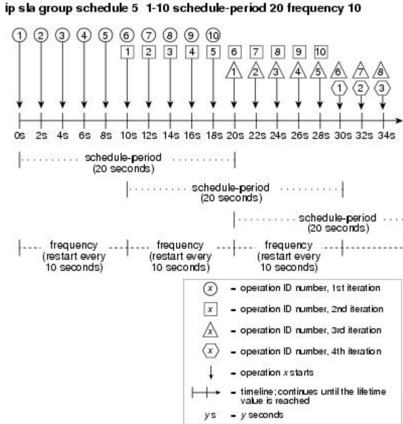
In this example, the first operation (operation 1) in operation group 5 will start at 0 seconds. All 10 operations in operation group 5 (operation 1 to operation 10) must be started in the schedule period of 20 seconds. The start time of each IP SLAs operation is evenly distributed over the schedule period by dividing the schedule period by the number of operations (20 seconds divided by 10 operations). Therefore, each operation will start 2 seconds after the previous operation.
