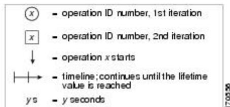
In this example, the first operation (operation 1) in operation group 1 will start at 0 seconds. All 10 operations in operation group 1 (operation 1 to operation 10) must be started in the schedule period of 20 seconds. The start time of each IP SLAs operation is evenly distributed over the schedule period by dividing the schedule period by the number of operations (20 seconds divided by 10 operations). Therefore, each operation will start 2 seconds after the previous operation.
