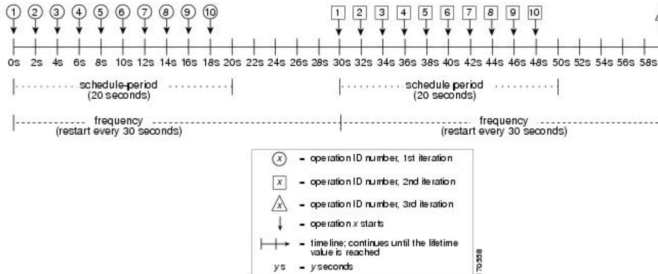
In this example, the first operation (operation 1) in operation group 2 will start at 0 seconds. All 10 operations in operation group 2 (operation 1 to operation 10) must be started in the schedule period of 20 seconds. The start time of each IP SLAs operation is evenly distributed over the schedule period by dividing the schedule period by the number of operations (20 seconds divided by 10 operations). Therefore, each operation will start 2 seconds after the previous operation.
