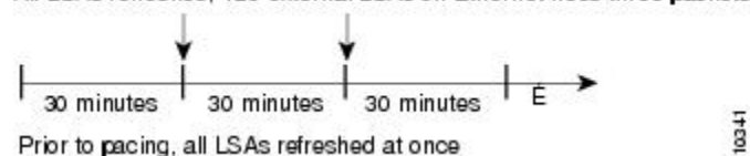
Figure 2 OSPF LSAs on a Single Timer Without Group Pacing
