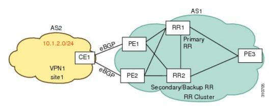
In the following configuration example based on the figure above, RR2 is configured with an additional path, which is a backup path.
