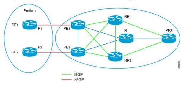
In the figure above, P1 and P2 are diverse paths for prefix p. Assume Path 2 (P2) has a lower MED and higher local preference than P1. The BGP Best External feature on PE1 will make sure that P1 is propagated to the
