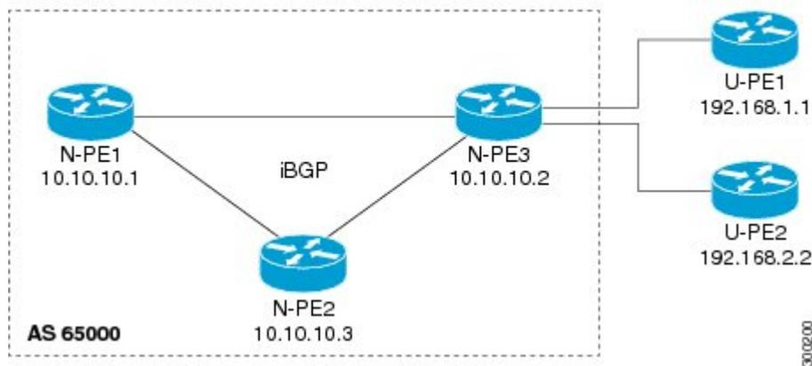
In this task, the PE router N-PE3 in the figure above is configured with a Layer 2 router ID, a VPN ID, a VPLS ID, and is enabled to automatically discover other PE routers that are part of the same VPLS domain. A BGP session is created to activate BGP neighbors in the L2VPN address family. Finally, two optional **show** commands are entered to verify the steps in the task.
