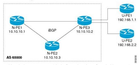
In this task, the PE router N-PE3 in the figure above is configured with a Layer 2 router ID, a VPN ID, a VPLS ID, and is enabled to automatically discover other PE routers that are part of the same VPLS domain. A BGP session is created to activate BGP neighbors in the L2VPN address family. Finally, two optional **show** commands are entered to verify the steps in the task.
