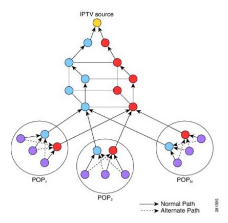
When a routing failure occurs, for example due to a link failure in the blue path, the red upstream router in the red plane becomes the primary upstream router to reach the source. This link to the router then becomes the RPF interface, and the copy of the multicast stream being received on the link is accepted and forwarded to the downstream links.
