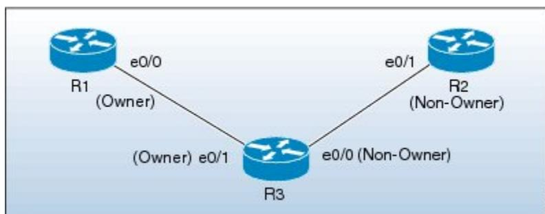
In this topology, device R3 is incorrectly inserted between the devices R1 and R2, with its interfaces swapped. The conflict arises due to incorrect insertion, as given below:
