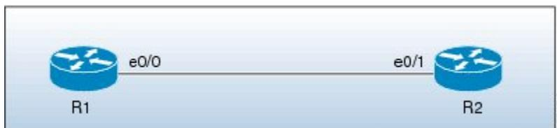
The e0/0 interface on device R1 is configured with the auto-IP address 10.1.1.1 and the e0/1 interface on device R2 is configured with the auto-IP address 10.1.1.3.
