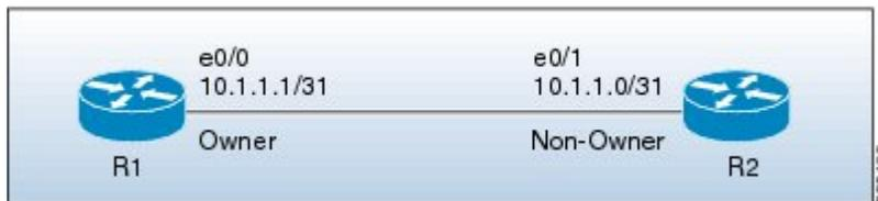
Device R1 is configured as the seed device. Interface e0/0 on R1 is configured with the IP address 10.1.1.1/31, and is the owner of the subnet connecting R1 and R2. Interface e0/1 on device R2 has the IP address 10.1.1.0/31, and is the non-owner interface of the subnet.
