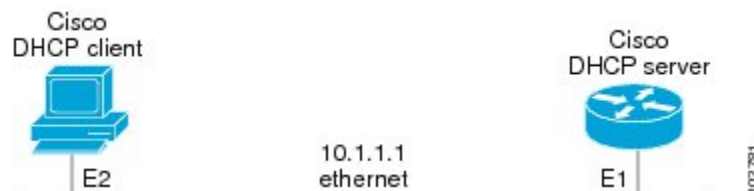
Figure 2 Topology Showing a DHCP Client with a Gigabit Ethernet Interface
