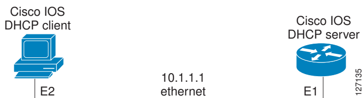
Figure 8 Topology Showing a DHCP Client with a Ethernet Interface
