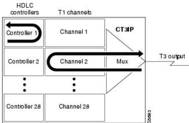
The figure below shows an example of a remote inband loopback in which the network line enters a line loopback.
