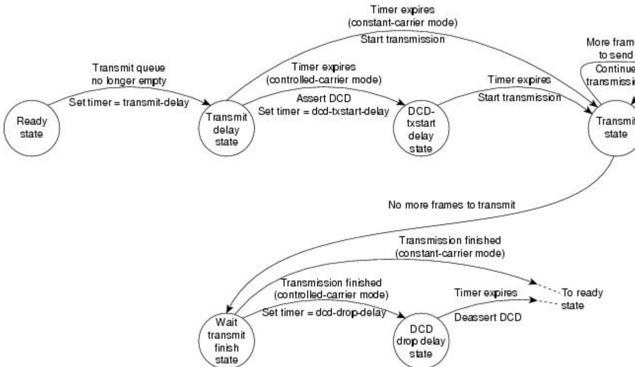
After the transmit delay state, the next state depends on whether the interface is in constant-carrier mode (the default) or controlled-carrier mode.
