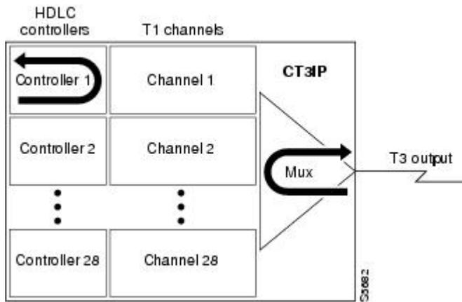
The figure below shows an example of a network payload loopback in which just the payload data is looped back toward the network at the T1 framer.
