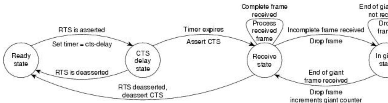
When the timer expires, the DCE state machine asserts CTS and transitions to the receive state. It stays in the receive state until there is a frame to receive. If the beginning of a giant frame is received, it transitions to the in giant state and keeps discarding all the fragments of the giant frame and transitions back to the receive state.
