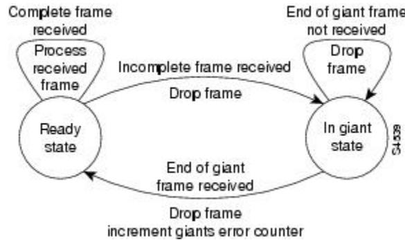
An error counter is incremented upon receipt of the giant frames. To view the error counter, use the **show interfaces** command for the serial interface in question.
