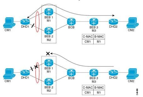
Device DHD1 is dual-homed to two 802.1ah backbone edge bridges (BEB1 and BEB2). Assume that initially the primary path is through BEB1. In this configuration BEB3 learns that the host behind DHD1 (with MAC address CM1) is reachable via the destination B-MAC M1. If the link between DHD1 and BEB1 fails and the host behind DHD1 remains inactive, the MAC cache tables on BEB3 still refer to the BEB1 MAC address
