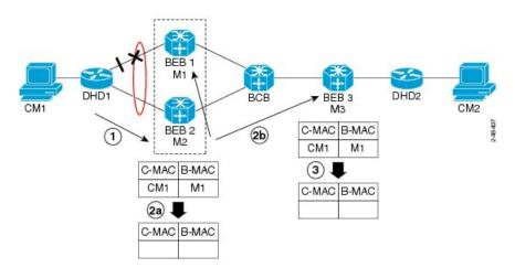
The MIRP has not been defined in IEEE but is expected to be based on the IEEE 802.1ak Multiple Registration Protocol (MRP). MRP maintains a complex finite state machine (FSM) for generic attribute registration. In the case of MIRP, the attribute is an I-SID. As such, MIRP provides a mechanism for BEBs to build and prune a per I-SID multicast tree. The C-MAC flushing notification capability of MIRP is a special case of attribute
