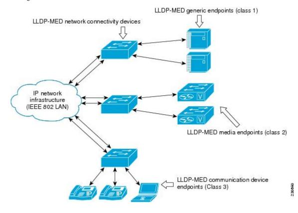
The figure below shows an LLDP-MED-enabled LAN.
