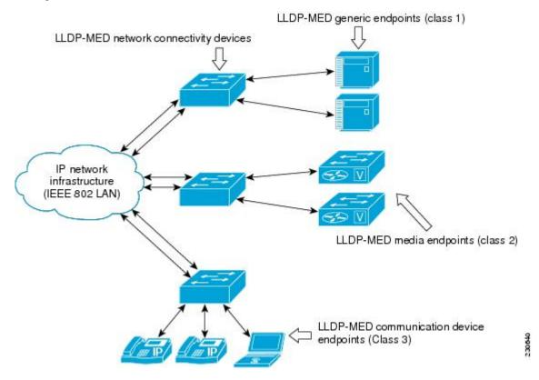
The figure below shows an LLDP-MED-enabled LAN.
