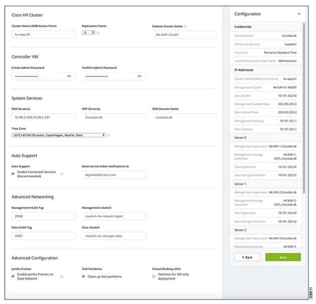
**Step 9** Click **Start** to begin the deployment. The **Progress** page displays the progress of the configuration tasks: Start, Deploy Validation, Deploy, Create Validation, Cluster Creation.
