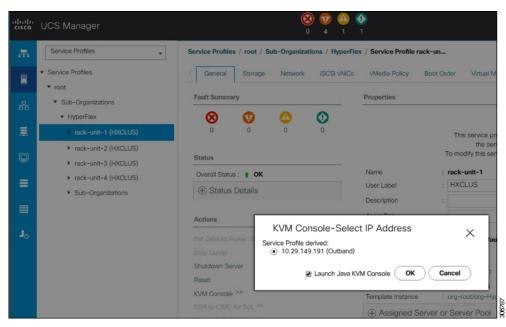
e) Reboot the host, launch the KVM Console, and power on the server to monitor the progress of the Windows installation. You should see the **Loading Files** screen appear. Windows should install automatically without user intervention.
