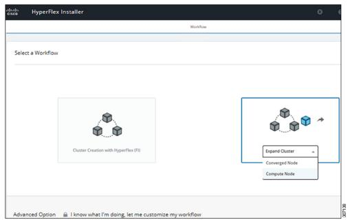
Step 4 In the Select a Workflow page, select Expand HX Cluster. Leave the Is OS installed on the Node, Run Hypervisor Configuration and Deploy HX Software checkboxes selected.
