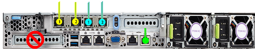
Intel X710 quad-port 10G / Cisco-Intel E810XXVDA4L 4x25/10G
