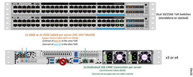
10/25 Gigabit Ethernet Single Switch Physical Cabling
