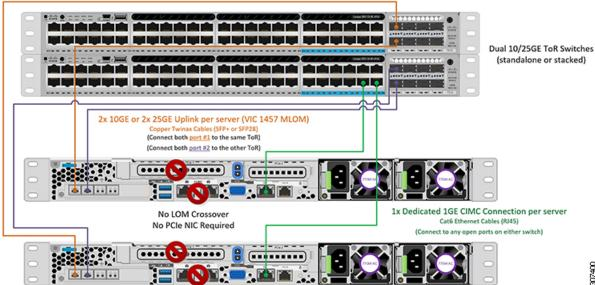
10/25 Gigabit Ethernet Single Switch Physical Cabling
