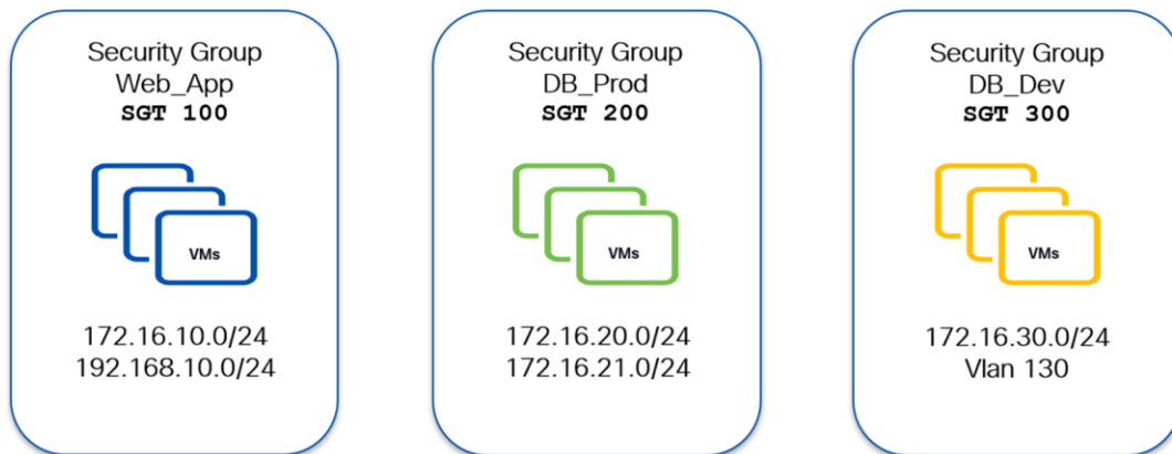
Figure 11. Network-Centric Approach for Security Group classification
