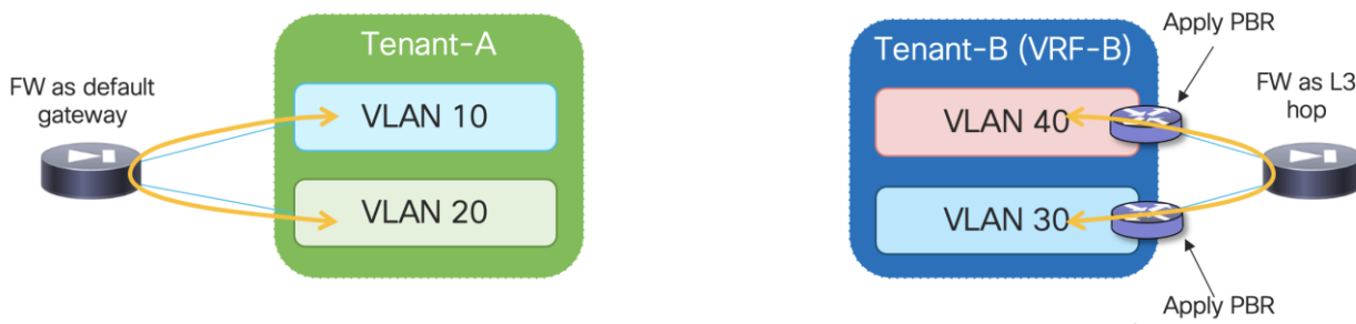
Figure 1. Intra-Tenant Security Enforcement
